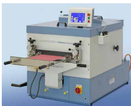
LABCOATER type «LTE-S», the optimum combination of dryer and laboratory coating table. Various kinds of material samples are coated in the same run and heat treated. The coating is applied either by floating, roller or rubber blanket knife. Multiple coatings which do not require re-loading are also possible.
