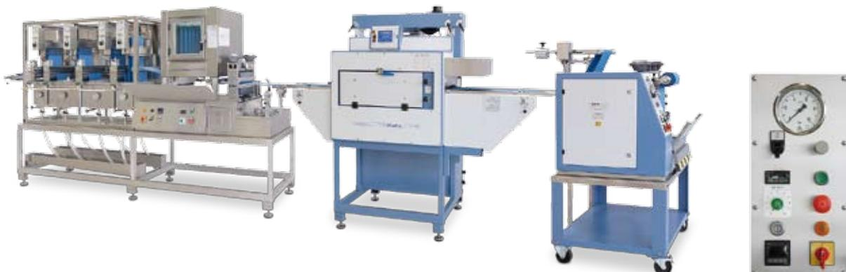
«HVF» – «KTF» – «TPS» combination for practical, continuous dyeing processes in the laboratory.
