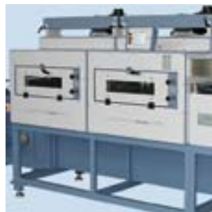
Double field dryer for different treating temperatures
