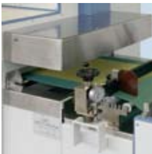
Infrared predryer for optimum heat pretreatment
