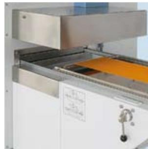
Infrared predryer for optimum heat pretreatment
