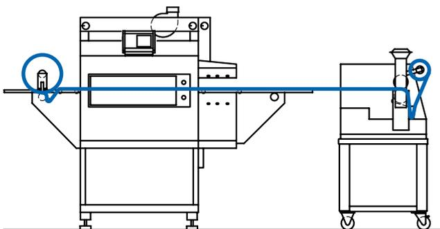
Continuous process flow in combination with MATHIS padder horizontal, vertical type «HVF»
