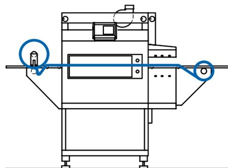
Continuous process flow from roll to roll
