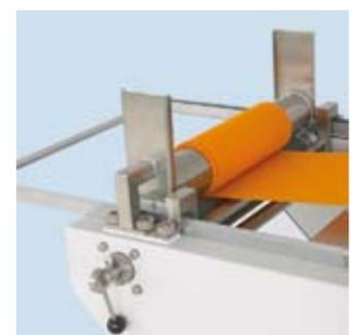
Upwinding device, designed as rising roll batcher
