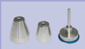
standard sample holder & 12 / 9 kPa load pieces
